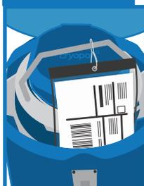
Remove the Leg 3 shipping pouch from the document protector attached to the dewar handle inside of the container.
