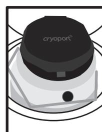
Close the hinged cap by pulling down on the lid. Let the shipper stabilize, undisturbed, for at least 30 minutes.
