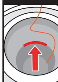
Slowly pour Liquid Nitrogen into opening. Fill the dewar up to the bottom of the neck tube.
