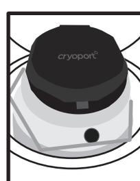
Close the hinged cap by pulling down on the lid. Let the shipper stabilize, undisturbed, overnight.
