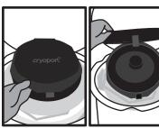
Open the hinged cap by pulling up on one of the two lift handles on the lid. With gloved hands, pull up on the circular handle in the center of the vapor plug to remove the vapor plug. Set the vapor plug aside.
