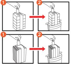
Open Bag and insert one rack into top opening. Lower rack completely into bag.
