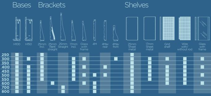
The depth of the shelves varies from 250+50 mm to 800+50 mm at 50 mm intervals, but for some types it is limited to less bulky sizes in order to maintain an acceptable load capacity. The table shows the complete range of bases, shelves and
