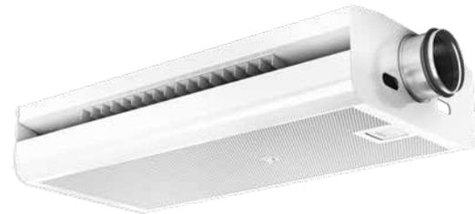
The room controller is integrated in the front plate of NOVA II and wired. This configuration uses the temperature sensor built into the room controller. Condensation sensor (in option) is factory wired.
