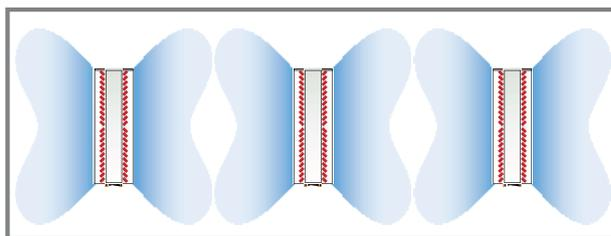
For high airflow applications as illustrated below, comfort control is in symmetrical setting, while FPC blades set at 30° angle settings on opposing units to avoid colliding air streams.
