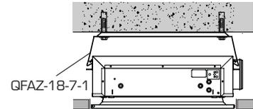
If there is a need for adjusting the installation height, suspension brackets and suspension rods M8 (QFAZ-12) can be ordered as well.
