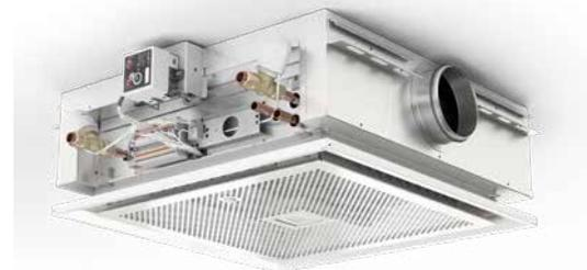
The room controller is factory mounted integrated in the front plate of LYRA II and wired. This configuration uses the temperature sensor built into the room controller. Condensation sensor (in option) is factory wired.
