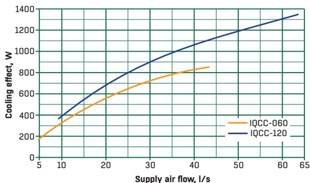
The diagram shows the approximate cooling power  $P_{tot}$  in W with water flow  $q_w = 0.05$  l/s, temperature difference between room air and supply air  $\Delta t = 8^\circ\text{C}$ . Temperature difference between mean water temperature and room temperature,  $\Delta t = 8^\circ\text{C}$ . Total air pressure drop 70 Pa.
