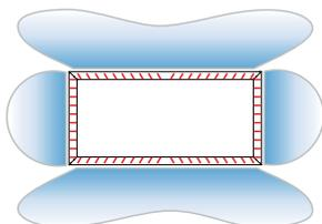
For high airflow applications as illustrated below, Energy Control is in symmetrical setting, while FPC blades set at 30° angle settings on opposing units to avoid colliding air streams.
