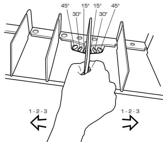
The image below shows an installation where air direction is set to 30 ° in two directions and the airflow is set with Energy Control to the same nozzle on each side of a size 120. This installation options provide an efficient and comfortable air throughout the room.
