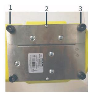
2. Pull the battery plate away from the device and disconnect the battery Molex. Release the battery from the battery holder by removing the Velcro strap. Install the new battery in the battery holder, reconnect the Molex connection, and secure the battery using the Velcro strap. Turn the device on and verify negative pressure from the vacuum tubing. Re-attach the battery plate to the base plate.
