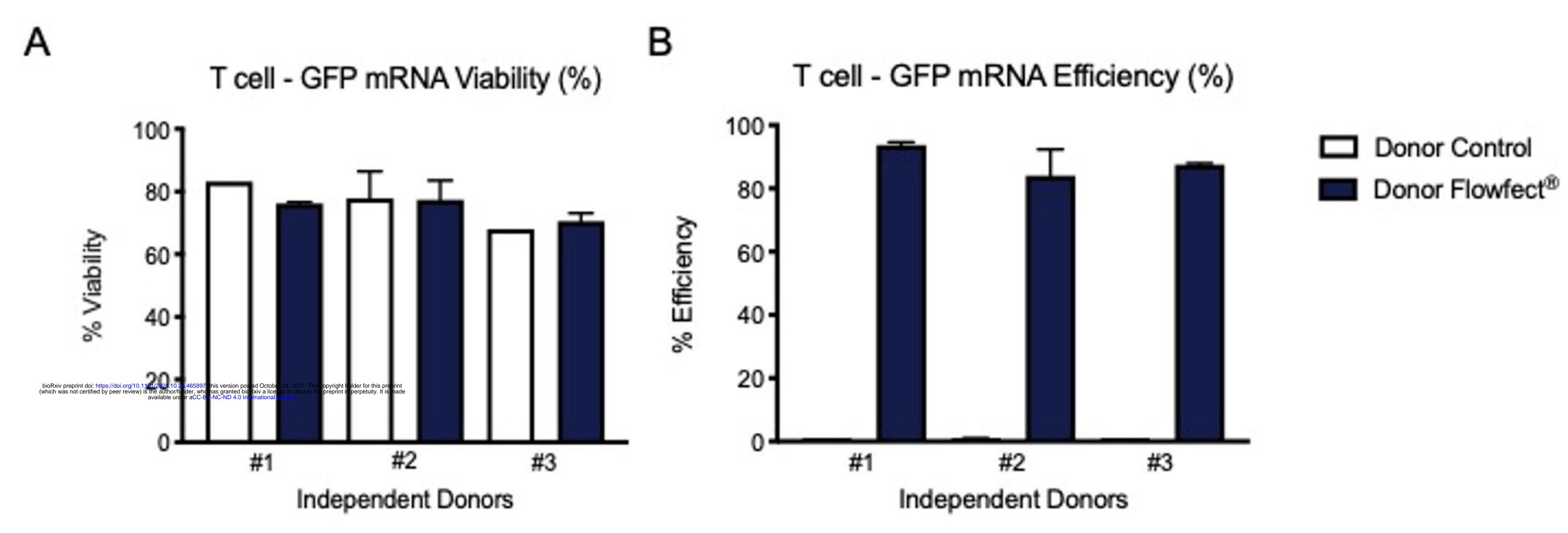
Fig. 4. Flowfect® technology can be used across different donors. Expanded human T cells from three unique donors were transfected with a GFP reporter mRNA using the Flowfect® Array platform. Cultures were assessed for A) cell viability (7AAD negative) and B) transfection efficiency at 24 hours. Bar graphs are Mean  $\pm$ SD with the following transfection sample sizes Donor #1 n=3 Donor #2 n=22 Donor #3 n=3.
