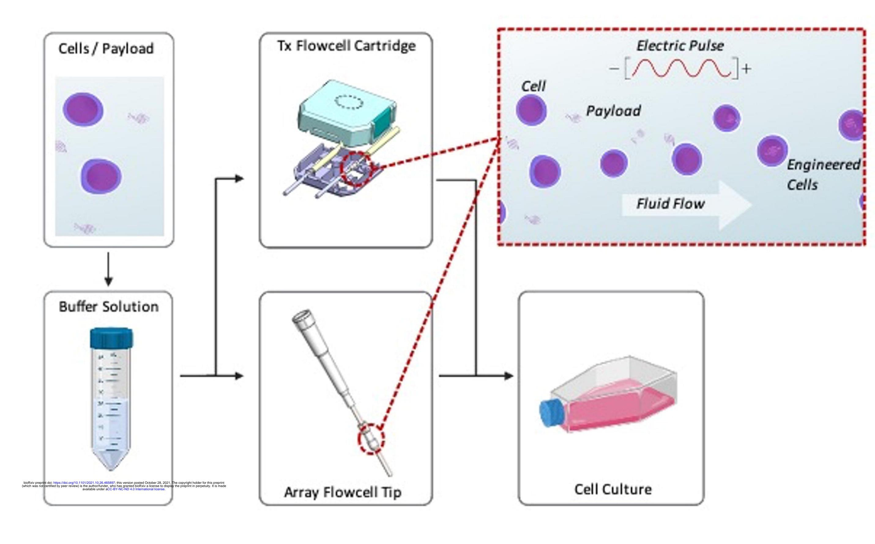
Fig. 1. Schematic of our continuous flow non-viral Flowfect® platform. Cells & payload are suspended in proprietary buffer in the reservoir. As the cells & payload flow through the electro-mechanical zone they are exposed to both electric field energy and continuous fluid flow to induce transient cell membrane disruption and simultaneous delivery of genetic payloads into the cells. Transfected cells are then dispensed directly into growth media for cell recovery.
