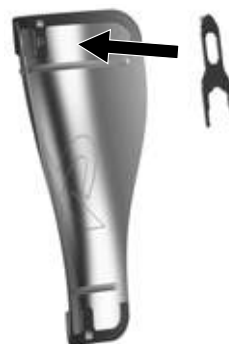
Fig. 10 Fitting adjusting fork F on the backside of coupling guard (7)
