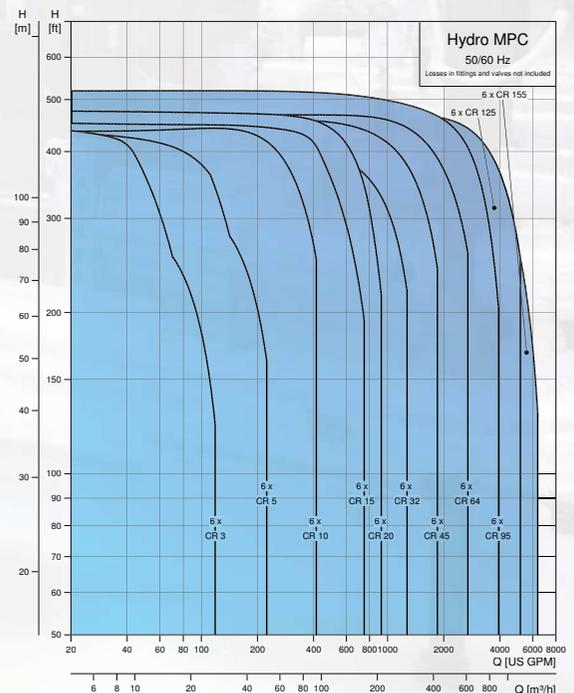
The Hydro MPC HVAC offers configurations to handle almost any head and flow, delivering consistent performance year after year.
