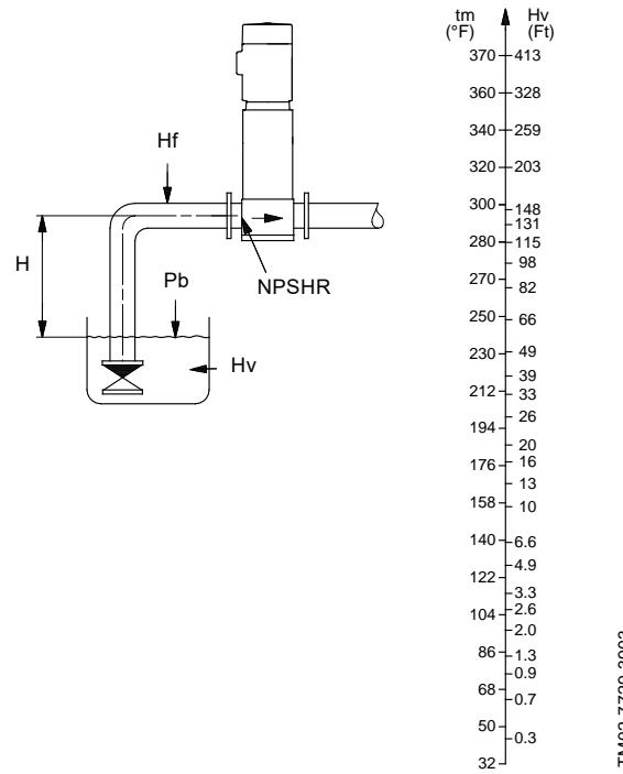
Fig. 15 Minimum inlet pressure - NPSHR
