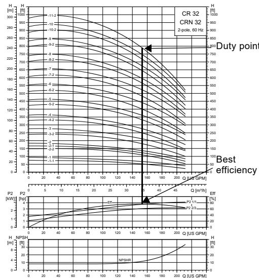
**Fig. 8** Example of a CR pump's duty point
