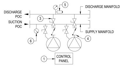
DUPLEX HYDRO CME BOOSTER PUMP DETAIL AND SCHEMATIC
