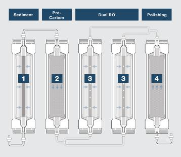
**Sediment Filter** Reduces particles such as dirt, silt, rust and pipe residue.
