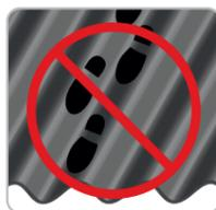
**4** Foot traffic on sheets should be kept to a minimum, whether on the ground, on the stack or fixed on the roof. Do not step on side lap corrugations
