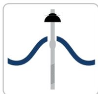
**6** It is recommended that a self-drilling top-fix screw is adopted. This simple operation offers a fast, low cost fixing solution. Using the correct Fibre Cement fixings with Reamer Wings on Shank, you can perfect the ideal fixing.
