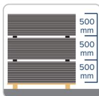
**6** If several stacks are to be laid one on top of the other, timber cross bearers should be placed at 500mm intervals up to a maximum height of 3000mm. It is important that the ground is level and firm.
