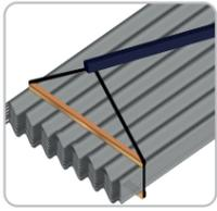
**1** The majority of deliveries in the UK are off-loaded by piggy-back fork lift. However subsequent crane handling should be careful to avoid damage to the edges of the sheets. Use rope slings (not chains) and over width spreaders to eliminate the possibility of damaging the edges of the sheets. The corners of the sheets are particularly vulnerable during any transportation period.
