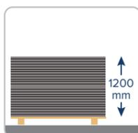
**5** Stacks without additional timber cross bearers should not exceed 1200mm. Cross bearers should be no more than 1 metre apart. Different length sheets should ideally be stacked separately but, if stacked with longer sheets, they must be laid on the top and their cross bearers must line up vertically.
