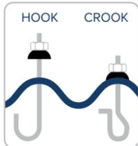
**5** Hook and crook bolts are commonly used to secure sheets. Clearance holes 2mm LARGER than the fixing should be pre-drilled to accept the fixing. The appropriate washer must be used to seal the operation.
