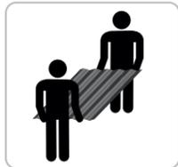
**3** If an onsite lift facility is unavailable, each sheet should be carefully removed by hand as described in 2. Once removed, they should be manoeuvred into position by two men at each end. Particular care should be taken in windy conditions.
