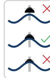
**2** To achieve a watertight and weathertight deal it is important to confirm that the sealing washer is correctly tightened. Not over-tight, nor too loose. After a period of time when the material has settled, the fixings may require re-tightening with hand tools. Be sure to use roof ladders to avoid walking on the sheets.
