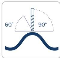
**4** Using a tungsten carbide tipped drill at a 90° angle to the sheet, drill a hole at least 2mm LARGER than the selected fixing diameter. The drill point should be no less than 60° to the sheet. Always drill at the 'apex' of the rise of a profile. Do not fix a sheet in the 'valley' or a 'slope' of the profile.
