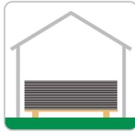
**1** Sheets and accessories should ideally be stored inside a building. Until the sheets are in position on the building they could be subject to damage from site debris and accidental collision. Rainwater, condensation and extreme weather conditions can also adversely affect the sheets (particularly coloured sheets) during this storage period. Ingress of moisture into packs of profiled sheets may cause efflorescence staining, bowing during installation or permanent distortion.
