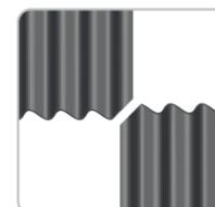
**3** To reduce the overlapping of four roof sheets, the corners of two must be mitred. Each mitre must be cut straight and cleanly either by hand or by power saw. The angle and size of the mitre is governed by the profile of the sheet and the end and side lap dimensions. Please ask for advice. It is recommended that a good quality butyl mastic strip is involved in the joining of the overlapping sheets to provide a weathertight seal.
