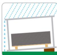
**3** If it is not possible to store the product inside a building, a suitable site should be selected. The ground should be firm and level and as close to the construction work as possible. The sheets must be stacked on cross bearers, thus raising them off the ground. A simple protective frame should be constructed and covered with a waterproof material. Air must be allowed to circulate all around the stack. The whole frame and stack should be tilted to encourage rainwater to drain freely.
