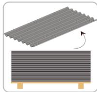
**2** Never push, drag or slide a sheet from the stack. Always consciously remove the sheets by lifting from the stack. Similarly lift the sheet into position a roof, do not push or drag over the purlins or other roof sheets.
