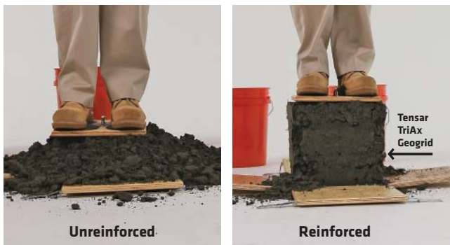
FIGURE 1 The lateral confinement of aggregate reinforcement with Tensor TriAx Geogrid is demonstrated through the box of rocks demonstration.
