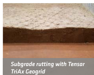
Testing using a small-scale trafficking device to compare the performance of Tensar TriAx and Tensar BX Geogrids.
