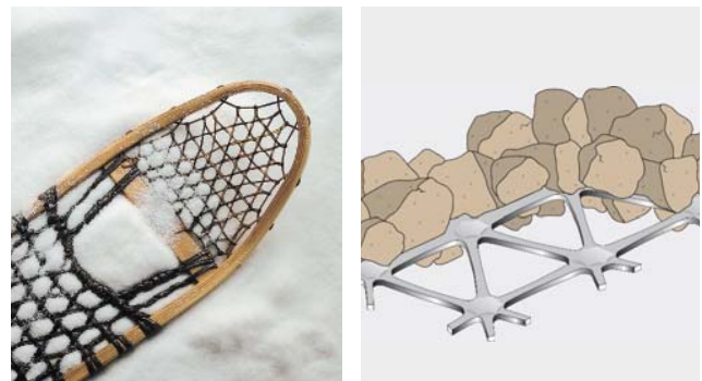
FIGURE 4 As a snowshoe distributes load over soft snow, Tensor TriAx Geogrid confines aggregate to better distribute in-service loads over soft subgrades.
