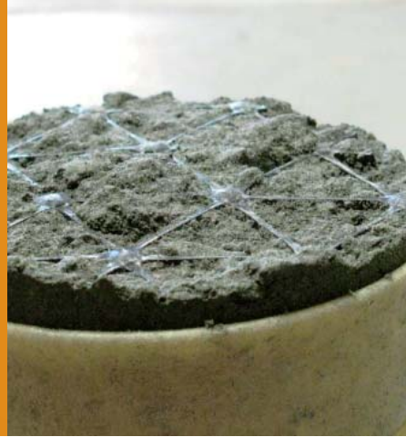
FIGURE 10 Small-scale research through a modified resilient modulus test confirms the stiffness enhancement achieved through the inclusion of a Tensar® TriAx® Geogrid within a crushed aggregate layer.
