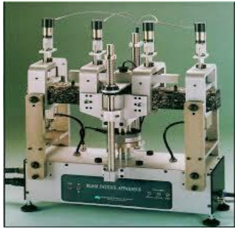
Fig. 25 – 4 Point Bending Beam Apparatus
