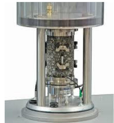
Fig. 30 – Typical AMPT Set Up
