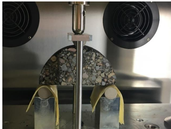
Figure 20 – SCB Test Set-up
