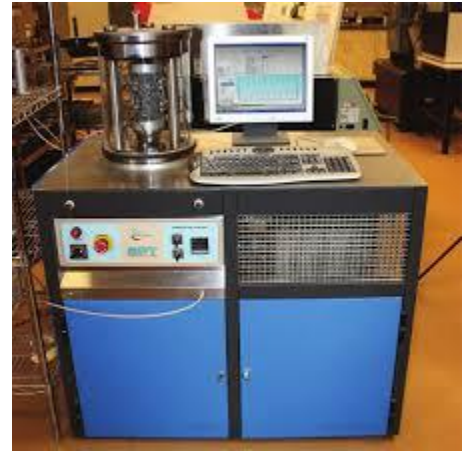
Fig. 29 – Typical AMPT Set Up
