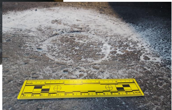
Figure 15 Permanent ACE Fiber Section Deformation after test completion
