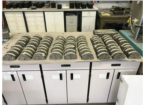
Figure 19 – SCB Test Samples
