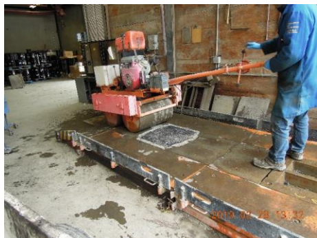
Fig. 26 – Preparation of Asphalt Concrete Beams
