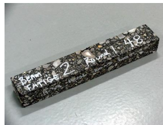
Fig. 27 – Typical Beam Test Sample
