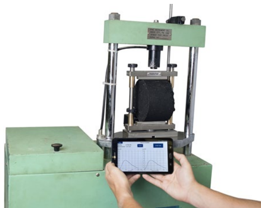
Figure 2. IDEAL-CT at Intermediate Temperature
