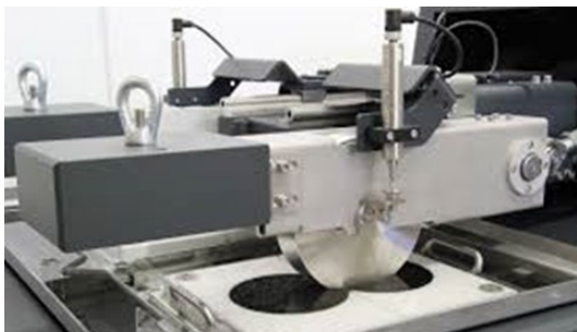
Figure 1. Hamburg Wheel Tracker (HWT) Test
