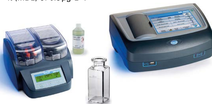
Figure 5: Combination reagent, digestion vials, and heater block (left), 1 in. (2.54 cm) sample cell (center), and spectrophotometer (right).
