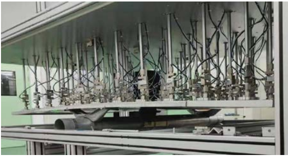
Load testing, such as Nextracker is undertaking in this image, can be key to ensuring a solar system is prepared for extreme wind events.
