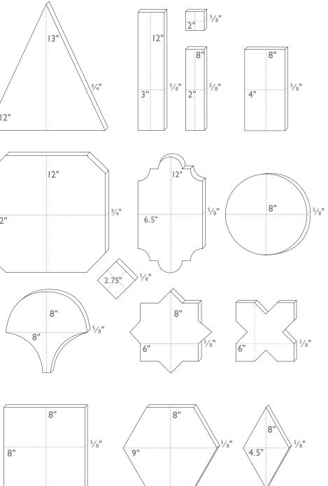
standard thickness for cement under 12" x 12" is  $\frac{5}{6}$ ". Standard thickness for cement over 12" x 12" is  $\frac{3}{4}$ ". Please note thickness can vary plus or minus  $\frac{1}{4}$ ".
