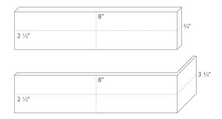
Standard thickness for Standard Issue bricks is  $\frac{1}{2}n^{****}$  and  $\frac{3}{4}n^{*****}$  for Forge bricks. 90° corner piece return is 3  $\frac{5}{6}n$  on Standard Issue and 3  $\frac{3}{4}n$  on Forge. Please note all dimensions are nominal and can vary plus or minus  $\frac{1}{4}n$ .
