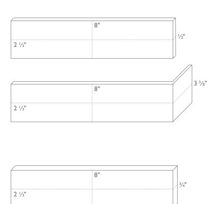
Standard thickness for Standard Issue bricks is ½"\*\*\*\* and ¾"\*\*\*\* for Forge bricks.
