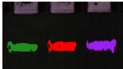
False color image of the same gel produced with Headwall's proprietary classification algorithm
