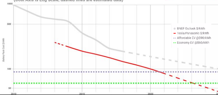
Trend Data for Battery Pack $/kWh - Tesla vs. Market Average (BNEF research) (Cost Axis is Log Scale, dashed lines are estimated data)
